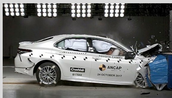
Frontal offset test at 64km/h
